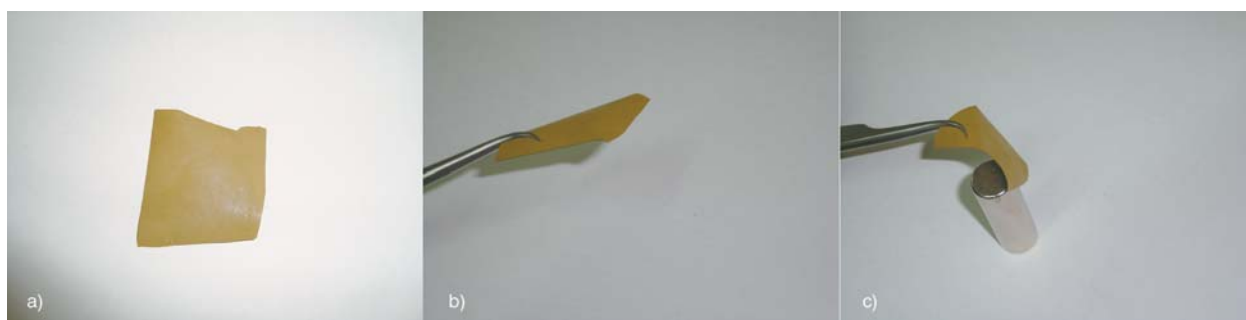
Figure 8. The Col 1:1 film (a) and the experiment carried out with a neodymium-iron-boron magnet; before (b) and after (c) magnetically attracted
