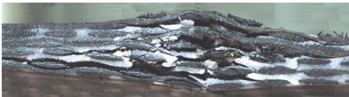
Figure 7. A typical 45° compressive shearing failure occurs in the compressive side of srPET composites accompany with fiber breakage, matrix crush, and delaminations
