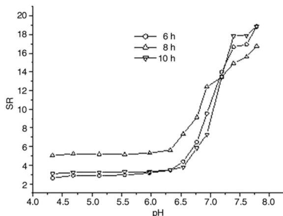
**Figure 8.** Effect of reaction time on pH-sensitivity of hydrogel
