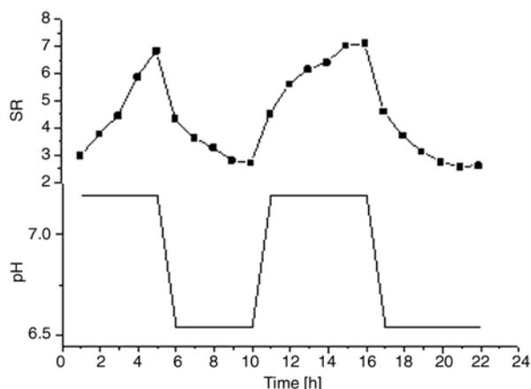
**Figure 11.** Swelling reversibility test of hydrogels as a function of time at 37°C under repeated changes in pH between 7.2 and 6.5
