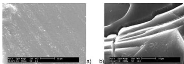
**Figure 6.** SEM images of blank hydrogels: a) the surface morphology; b) the cross-sectional view
