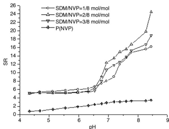
**Figure 9.** Effect of different amount of monomers on pH-sensitivity of hydrogel
