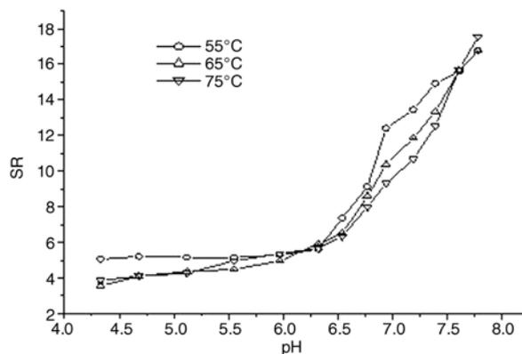
**Figure 7.** Effect of temperature on pH-sensitivity of hydrogel
