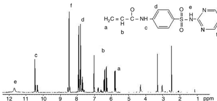
**Figure 5.**  $^1H$  NMR spectrum of sulfadiazine monomer in DMSO- $d_6$
