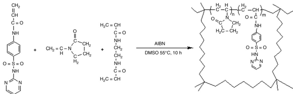
**Figure 3.** Chemical structures of gel components and the synthetic route of the hydrogel
