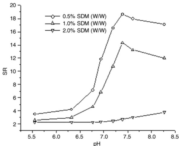
**Figure 10.** Effect of amount of cross-linker on pH-sensitivity of hydrogel
