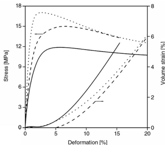
**Figure 1.** Stress vs. strain and volume strain traces of PE composites containing 20 vol%  $\text{CaCO}_3$  filler. — PE04, --- PE07, ····· PE11
