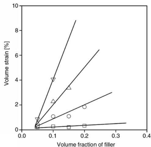
**Figure 11.** Volume increase in PE07 composites at different filler contents and deformation. Symbols: (□) 5%, (○) 10%, (Δ) 15%, (∇) 20% strain
