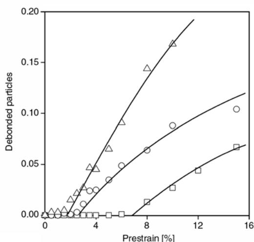
**Figure 5.** Effect of prestrain and matrix stiffness on the amount (in absolute volume fraction) of debonded filler in PE/CaCO<sub>3</sub> composites containing 20 vol% filler. (□) PE04, (o) PE07, (Δ) PE11
