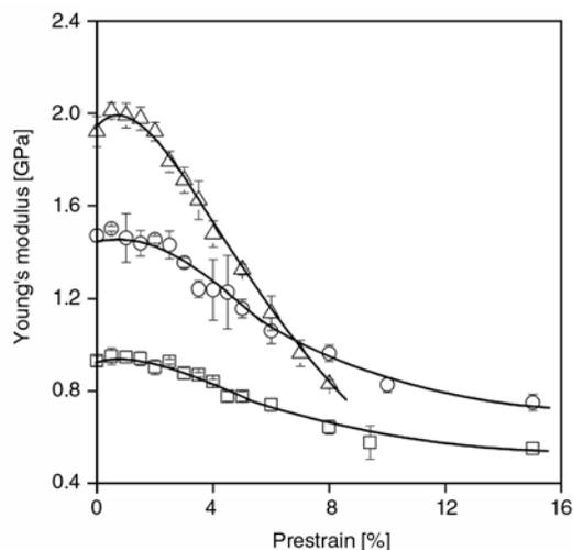
**Figure 4.** Dependence of the modulus of PE composites containing 20 vol% filler on the extent of prestrain. Symbols: (□) PE04, (○) PE07, (Δ) PE11
