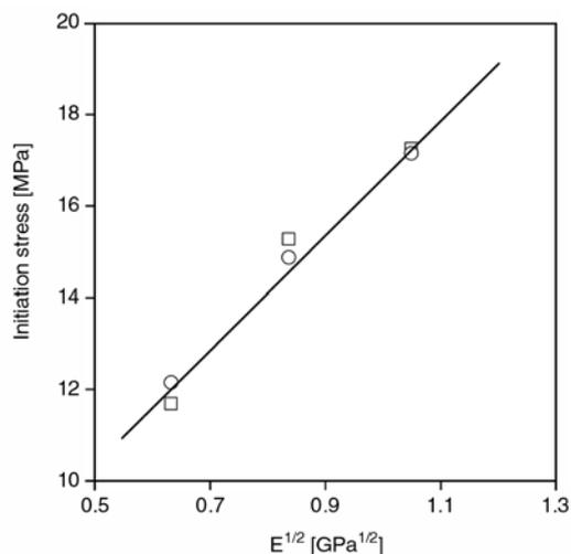
**Figure 2.** Dependence of debonding stress derived from the volume strain measurements on the stiffness of the matrix (see Equation (1)). Symbols: (□) 15 vol%, (○) 20 vol% filler
