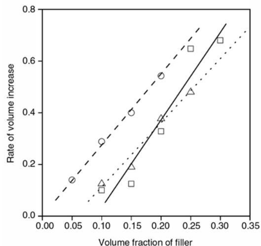
**Figure 8.** Effect of filler content and matrix stiffness on the rate of volume increase in PE/CaCO<sub>3</sub> composites. Symbols: ( $\square$ ) PE04, ( $\circ$ ) PE07, ( $\Delta$ ) PE11
