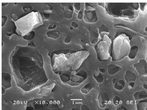
**Figure 7.** Size and shape of voids forming during elongation in PE/CaCO<sub>3</sub> composites; 5 $\epsilon_y$  strain
