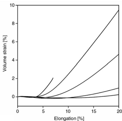
**Figure 3.** Effect of filler content on volume increase in PE04/CaCO<sub>3</sub> composites. Filler content increases from 0.1 to 0.3 volume fraction in 0.05 volume fraction steps from right to left
