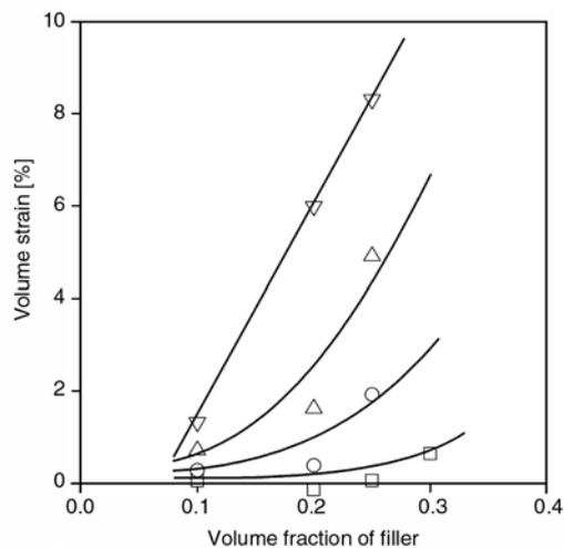
**Figure 10.** Effect of filler content and strain on volume increase; extensive plastic deformation during the elongation of PE04 composites. Symbols: (□) 5%, (○) 10%, (Δ) 15%, (∇) 20% strain
