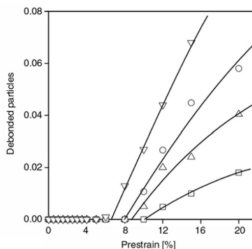
**Figure 6.** Influence of filler content on the number of debonded particles (in absolute volume fraction) in PE04/CaCO<sub>3</sub> composites. Symbols: (□) 5 vol%, (Δ) 10 vol%, (o) 15 vol%, (∇) 20 vol% filler
