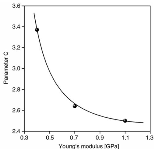
**Figure 9.** Dependence of parameter  $C$  on the stiffness of the matrix polymer
