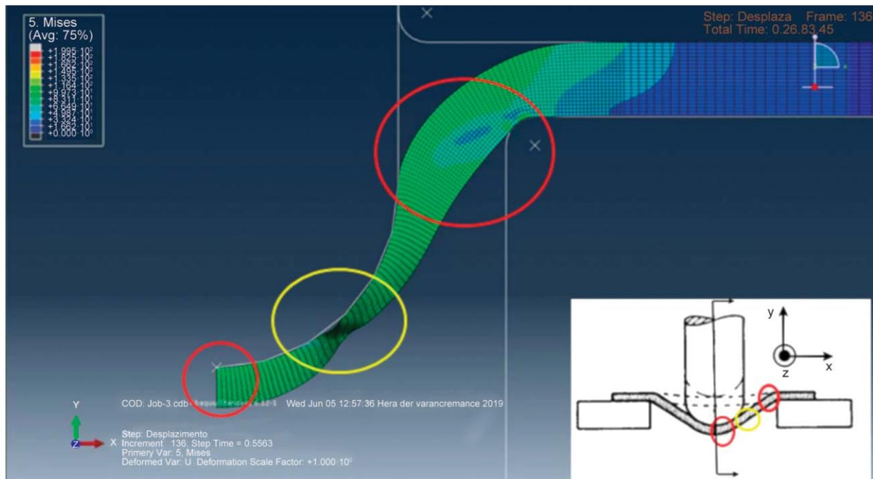
**Figure 7.** Image taken from a preliminary numerical simulation of the SPT test in EVOH, as an example of ductile behaviour in tensile test. Inset: Simplified scheme of the loading geometry and regions taken for monitoring the stress field involved during SPT.
