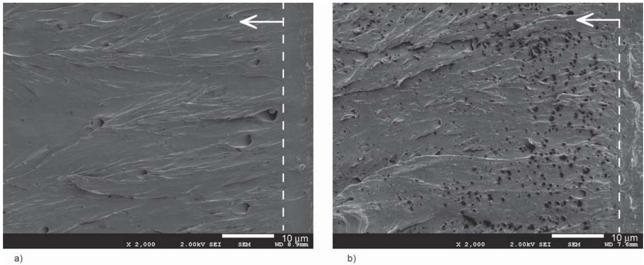
**Figure 5.** SEM micrographs of fracture surfaces taken from sharp-notched dumbbell tensile tests of: a) PLA/CNC and b) PLA/mCNC. Dashed line indicates the sharp-notch edge. Crack growth direction pointed with arrows.
