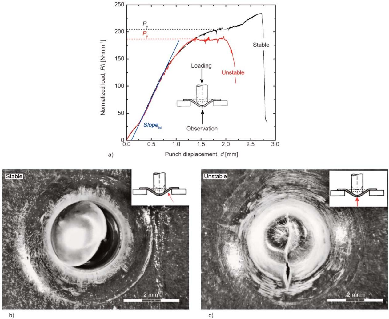
**Figure 6.** a) Representative thickness normalized load – punch displacement curves obtained for unstable and stable-ductile behaviour in PLA/mCNC. Inset: Simplified scheme of the loading solicitation mode during SPT. b) and c) optical micrographs of the tested samples with stable-ductile behaviour in PLA and unstable-ductile behaviour in PLA/mCNC, respectively. In upper right corner it is pointed with the arrow the location of the crack.
