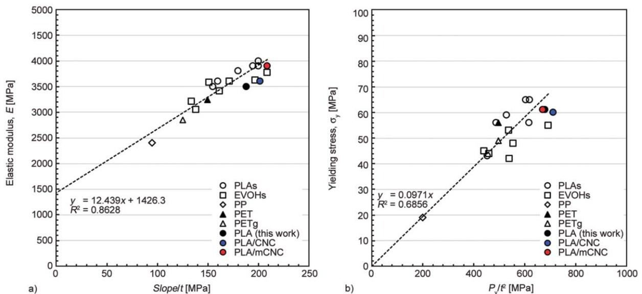
**Figure 8.** Graphical correlation between SPT and tensile parameters: a)  $Slope_{ini}/t$  vs.  $E$  and b)  $P_y/t^2$  vs.  $\sigma_y$ . Filled circles correspond to materials of this work (PLA in black, PLA/CNC in blue and PLA/mCNC in red). Other polymeric materials data are taken and adapted from [12].
